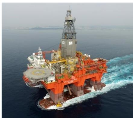
Semi-submersible rigs operate in both the midwater-, deepwater- and ultra-deepwater areas globally, depending on how the specific rig is dimensioned and equipped. Due to the good motion characteristics of Semi-submersibles, these rigs are the preferred floater type that operate in harsh environment areas. (See section 7.4 – “The Harsh Environment Segment” below).
