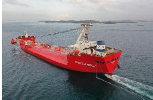
HTVs are used to carry project cargoes which do not fit into the holds of a conventional cargo ship. The loads are typically extremely large and heavy constructions. The HTVs operate in multiple markets, including the offshore wind, oil and gas, marine, dredging, and heavy construction markets.
