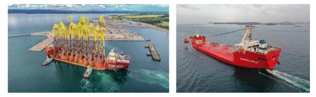
HTVs are used to carry project cargoes which do not fit into the holds of a conventional cargo ship. The loads are typically extremely large and heavy constructions. The HTVs operate in multiple markets, including the offshore wind, oil and gas, marine, dredging, and heavy construction markets.
